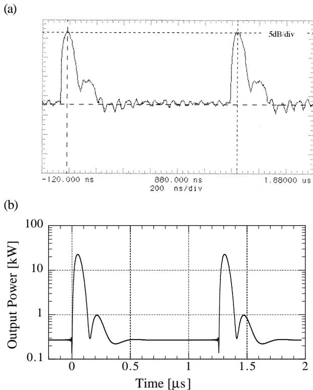
Fig.2 Output of the c-cavity with a current of 100mA single bunch. (a) is the measurement and (b) is the simulation.
