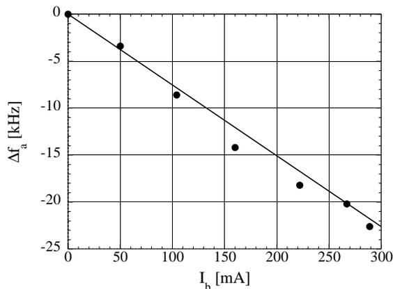
Fig.1 Frequency detuning of the a-cavity as a function of the beam current. The dots are measured value and the straight line is the expected value.
