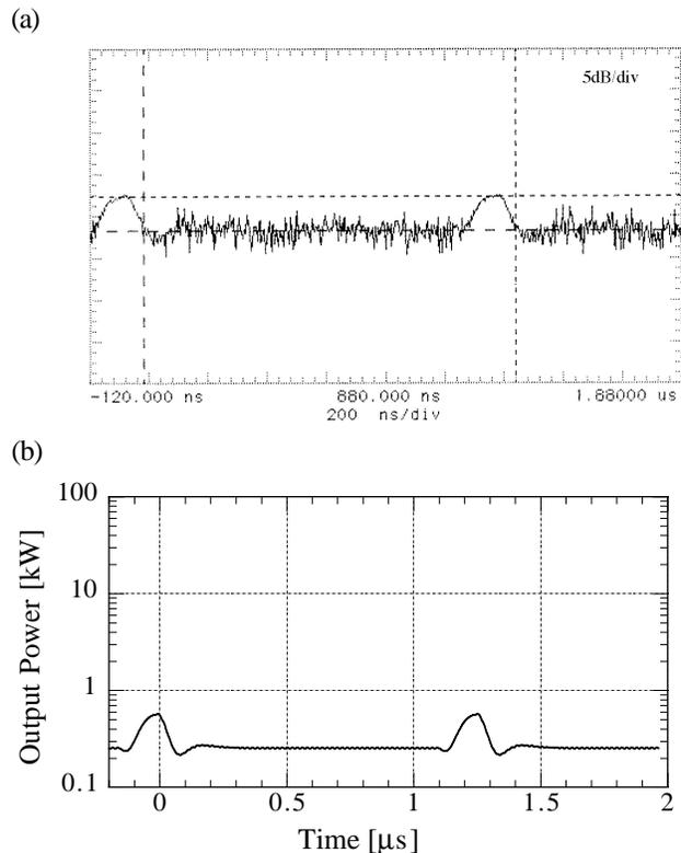
Fig.3 Output of the c-cavity when consecutive 56 buckets are filled out of equally spaced 64 buckets. The current was 164mA. (a) is the measurement and (b) is the simulation.
