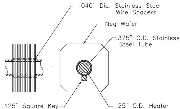
Fig. 2. Cross-section of a PEP-II NEG Pump
