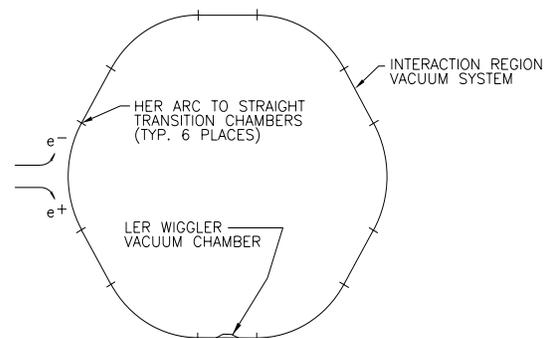
Fig. 1. NEG Pump Locations within the PEP-II B Factory
