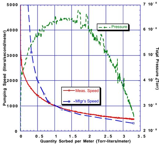
Fig. 4. Sorption Curve for a PEP-II NEG Pump
