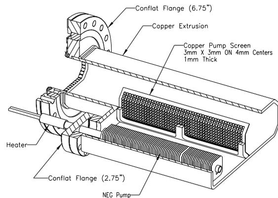
Fig. 3. NEG Pump in an IR Chamber
