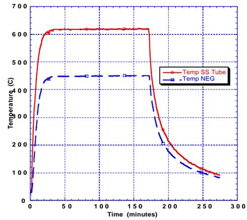
Fig. 5. Temperature Plot of Typical NEG Activation
