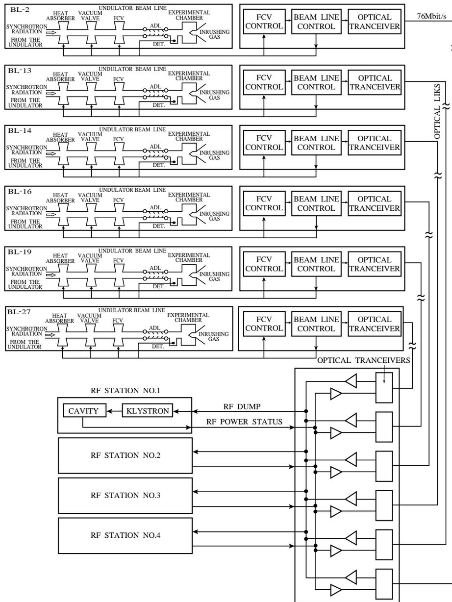
Figure 1 Block diagram of the Ultra-High-Vacuum protection system for synchrotron radiation beam lines with multiple wigglers and undulators
