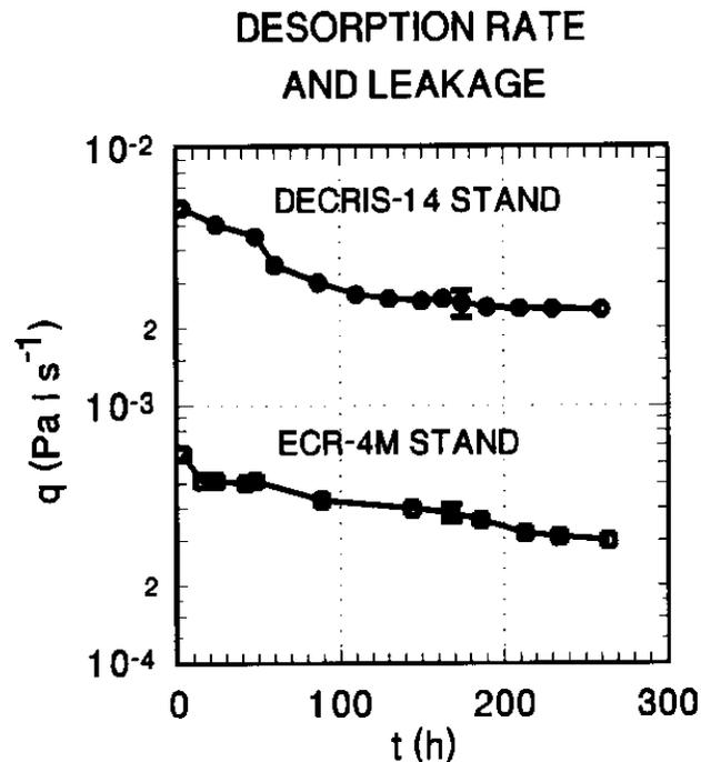
Figure 1: Measured desorption rates and leakages  $q$  of the DECRIS-14 and the ECR-4M vacuum stands as a function of pumping time  $t$ .
