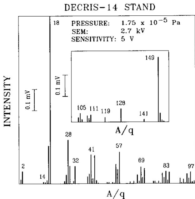
Figure 2: Measured mass spectrum of the residual gases from the DECRI-14 vacuum stand.
