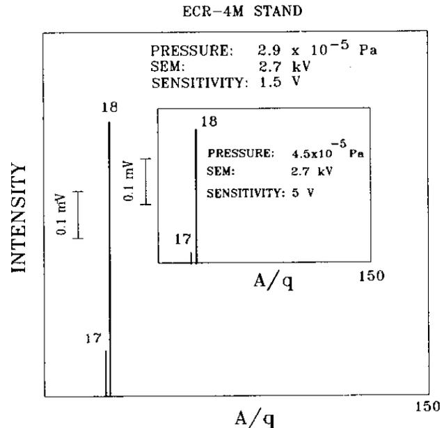
Figure 4: Other measured mass spectrum of the residual gases from the ECR-4M vacuum stand.
