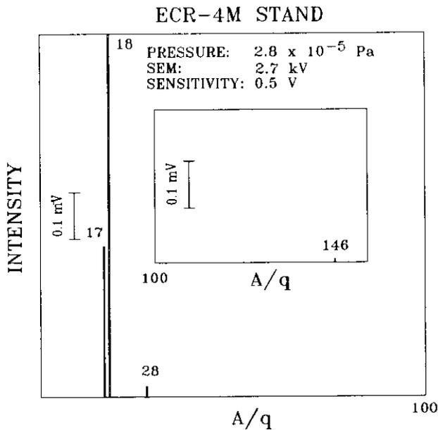
Figure 3: Measured mass spectrum of the residual gases from the ECR-4M vacuum stand.
