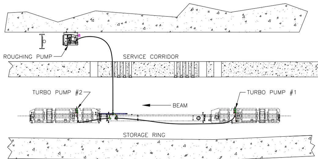
Figure 1: APS storage ring with ancillary pumping system.
