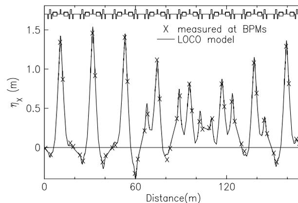
Figure 2: After the model was fit to the measured response matrix, the model also accurately predicted the measured  $\eta_x$ .
