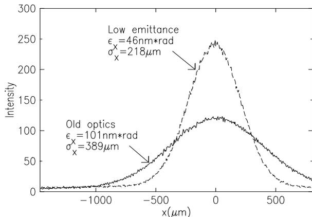
Figure 3: The reduction in X-Ray Ring horizontal beam profile as measured by an x-ray pinhole camera.
