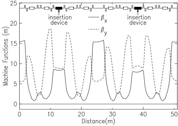
Figure 7: The  $\beta$ -functions in the NSLS VUV Ring did not have the design four-fold periodicity.
