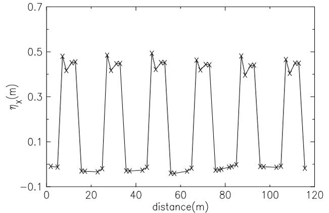
Figure 10: Measured  $\eta_x$  at SRRC after correcting for the BPM gain errors derived by analyzing the response matrix.
