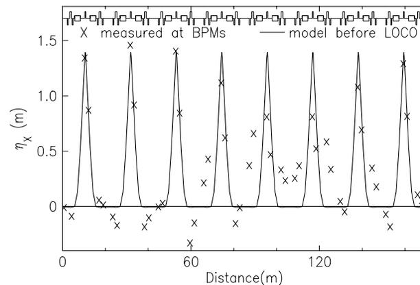
Figure 1: Before applying LOCO in the X-Ray Ring, the measured  $\eta_x$  differed significantly from the model.
