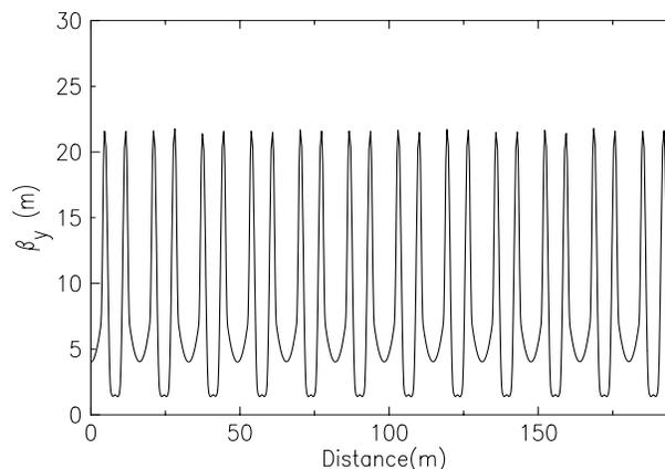
Figure 6: ALS vertical beta after correction with LOCO.
