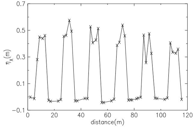
Figure 9: Measured  $\eta_x$  at SRRC without BPM gain error correction.
