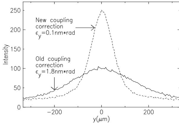
Figure 11: The reduction in X-Ray Ring vertical beam profile as measured by an x-ray pinhole camera.
