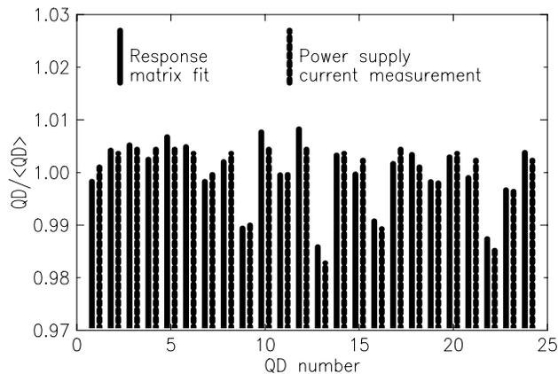
Figure 5: The variation in the fit gradients in the 24 QD quadrupoles agreed with the subsequent measurement of the current to each QD.
