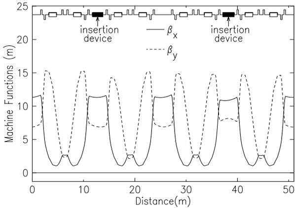
Figure 8: LOCO was able to find a set of quadrupole strengths that very nearly restored the design periodicity of the VUV Ring despite the strong vertical focusing of the insertion devices.
