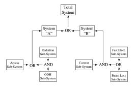
The purpose of the system picture is to logically group components of the system into blocks. These major blocks are used to determine the final system reliability. Each of the major sub-systems under investigation is further broken down into its sub-systems and components.
