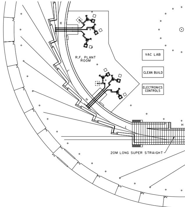
Figure 1. Layout of DIAMOND Storage Ring showing RF System Configuration.
