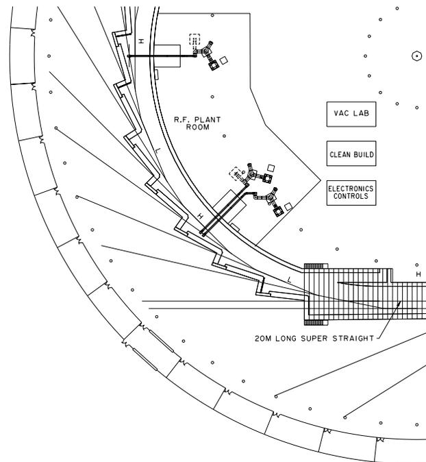
Figure 3. Layout of DIAMOND Storage Ring showing Superconducting Cavity Option.
