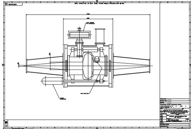
Figure 2. 350 MHz Superconducting Cavity in Cryostat
