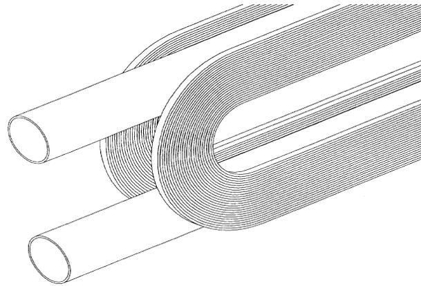
Fig. 1: The main coils in the 2-in-1 common coil design concept. The coils on the left and on the right sides of the beam tubes are common to both top and bottom apertures.
