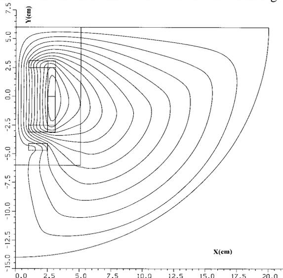
Fig. 3: The field lines at 15 tesla field in the lower-right quadrant of the proposed common coil design magnet. The coldmass is shown in  $\sim 1/3$  scale.
