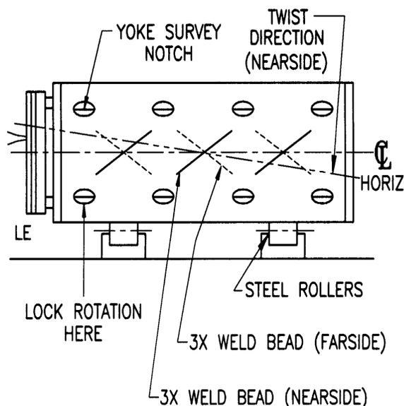
Figure 1. Schematic showing the procedure used to remove axial twist.
