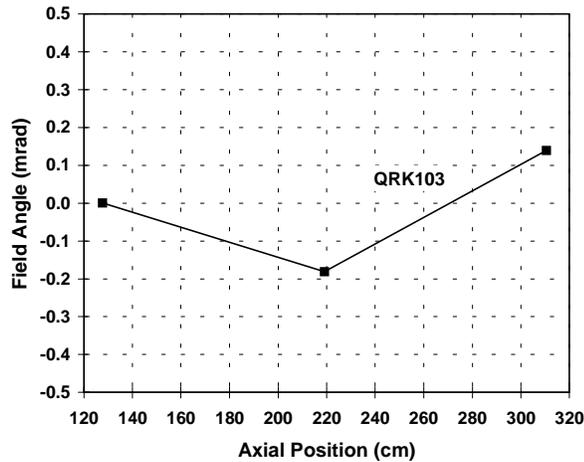
Figure 4. Field angle measured with a 0.91m long rotating coil at three axial locations in the straight section of the Q2 magnet QRK103.
