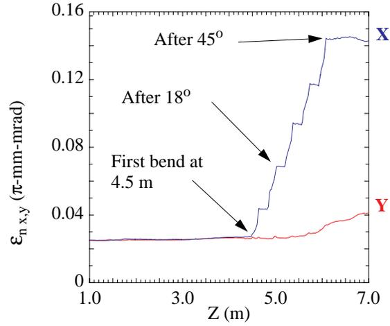
Figure 1: Normalized emittance at mid-pulse as the beam moves along the accelerator. The rise in the  $x$  emittance is due to the axial thermal spread of the beam in the bend. The  $y$  emittance begins to rise to match  $x$ . The thermal spread is 0.22% of the beam velocity.
