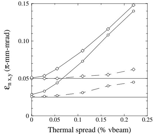
Figure 3: Final normalized emittance of the beam mid-pulse with changing axial thermal spread for two different initial emittances, 0.025 and 0.05  $\pi$ -mm-mrad. Solid line is in the plane of the bend, dashed is out of plane. The horizontal lines show the initial emittance. Comparison with the emittance from the experiment will give an indirect measurement of the axial thermal spread.
