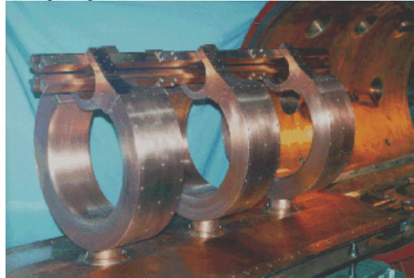
Figure 1. Photograph of the three modules ready to be installed in the tank.
