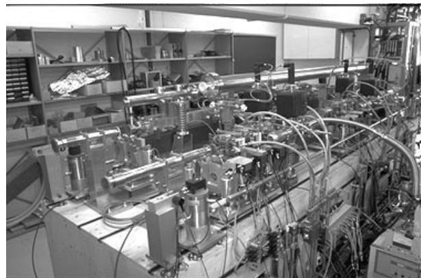
Figure 5: Pre-assembly of CTF2 30 GHz modules
