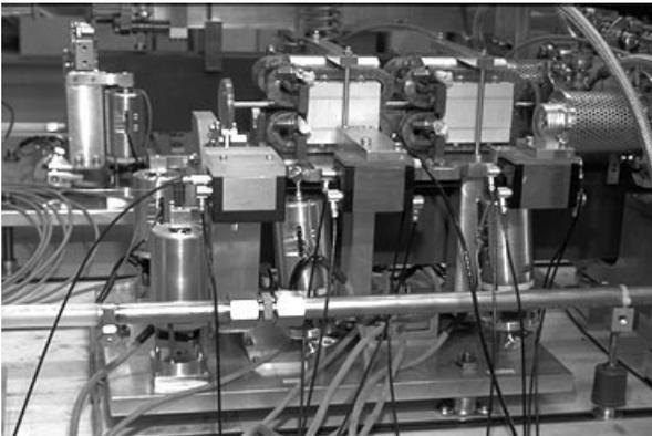
Figure 4: Quadrupole support
