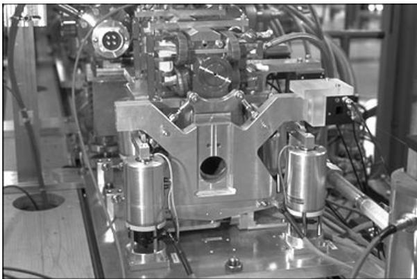
Figure 1: Inter-girder connection
