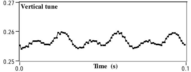
Fig.4 Modulation of vertical tune
