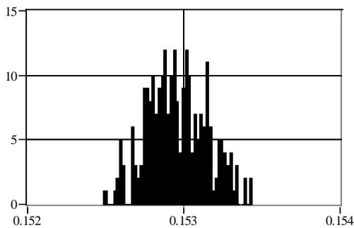
Fig.3 Distribution of horizontal tunes at 0 amplitude measured over 5 min. period at fixed phase relative to AC.
