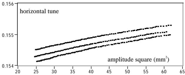
Fig.2 Horizontal tune vs. amplitude square for 3 consequent kicks.
