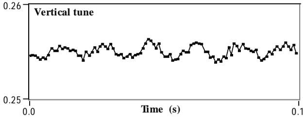
Fig.7 Modulation of vertical tune , no 30Hz power line interference
