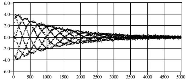
Fig.1 Horizontal centroid position (mm) vs. turn number
