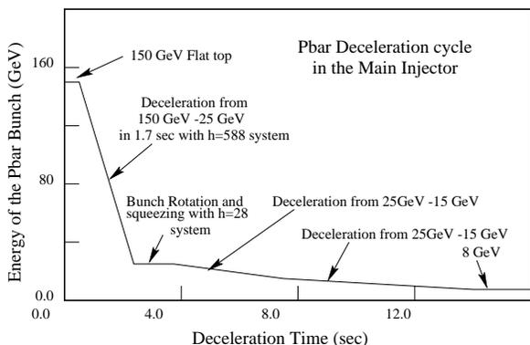
Figure 3: A 12.5 sec long  $\bar{p}$  Deceleration cycle used for simulation.
