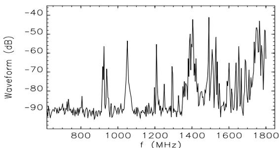
Figure 4: RF cavity HOM spectrum for stable beam.
