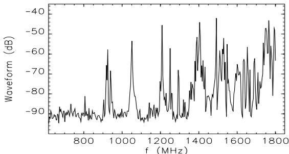
Figure 5: RF cavity HOM spectrum for unstable beam.
