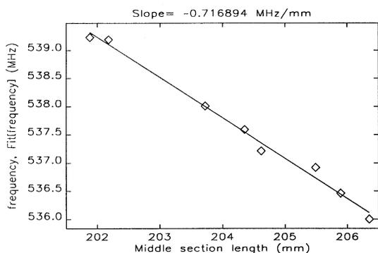
Figure 1: Cavity staggering effect at 536 MHz.
