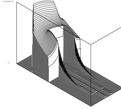
Figure 2: Magnetic field inside cavity and housing.
