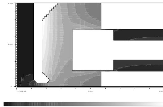
Figure 1: The magnetic field distribution in the cavity with the plunger.
