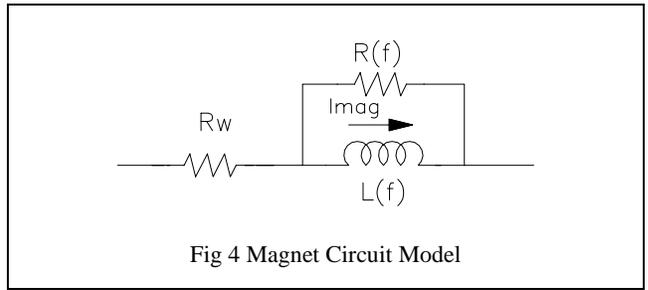
Fig 4 Magnet Circuit Model
