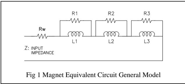
Fig 1 Magnet Equivalent Circuit General Model
