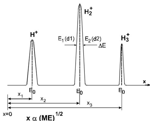
Figure. 5 The axial energy spread is found from the ion species traces. The energy of the individual ion peaks is the same and the distances are proportional to  $(ME)^{1/2}$ . The position of the individual ion peak center is the average energy of the extracted ion beam species.
