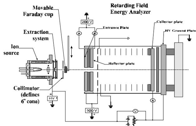
Figure. 3 Schematic of the retarding field energy analyzer system for accelerated beam energy spread measurements.
