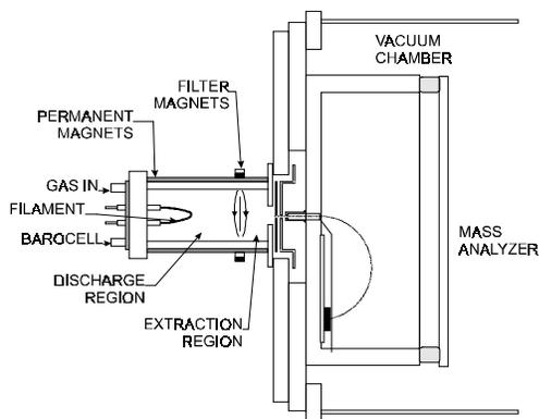
Figure. 4 Schematic drawing of a filament operated multicusp ion source mounted in a vacuum chamber. A magnetic analyzer is used for analyzing the collimated and accelerated beam.
