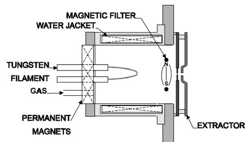
Figure. 1 Schematic of a multicusp ion source when is operated with a filament cathode.
