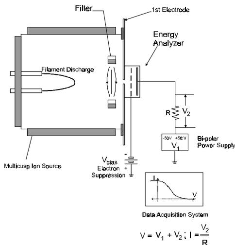
Figure. 2 Schematic of the ion source with the removable filter and the retarding field energy analyzer at the source aperture assembly.
