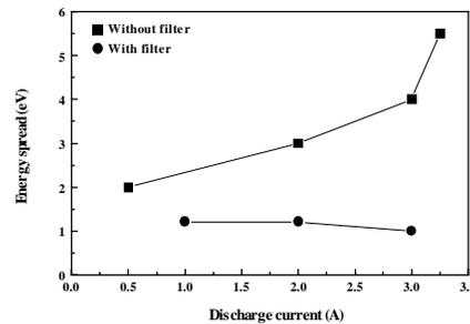
Figure. 9 Discharge current vs. energy spread for a 10 cm diameter source with and without a filter.
