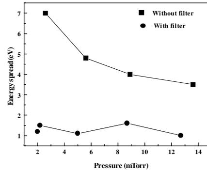
Figure. 8 Pressure vs. energy spread for a 10 cm diameter source with and without a magnetic filter.
