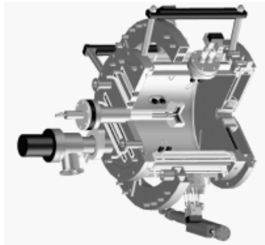
Figure 1: The LANSCE upgrade source. Shown here is the plasma chamber with the magnets and the filaments. The converter is mounted to the end plate. In the front
