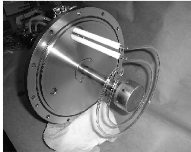
Figure 5: The endplate of the source with the quartz RF antenna. Note that a silver plated copper wire is inside the quartz tube. The antenna is water-cooled. Also shown is the converter.
