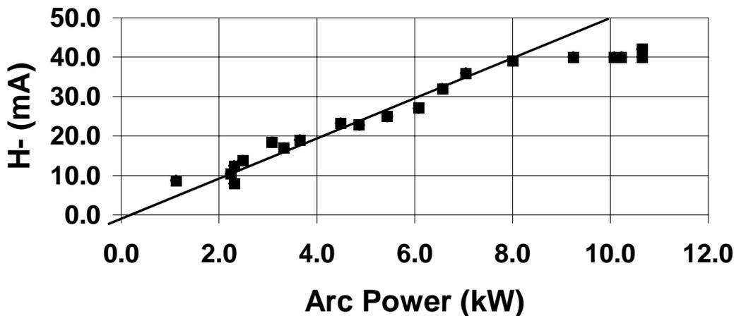
Figure 3: H<sup>-</sup> current as a function of discharge power. The arc and converter voltages are 70 and 300 V, respectively. The pulse length and repetition rate are kept constant at 1.2 ms and 100 Hz (12% duty factor), respectively. The cesium coverage is optimized by adjusting the converter surface temperature.
