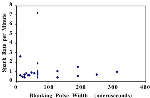
Figure 8: Spark rates as a function of blanking width.
