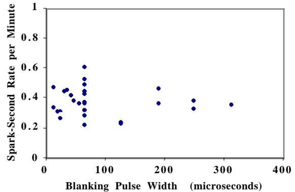
Figure 9: Spark-second rates as a function of blanking width.
