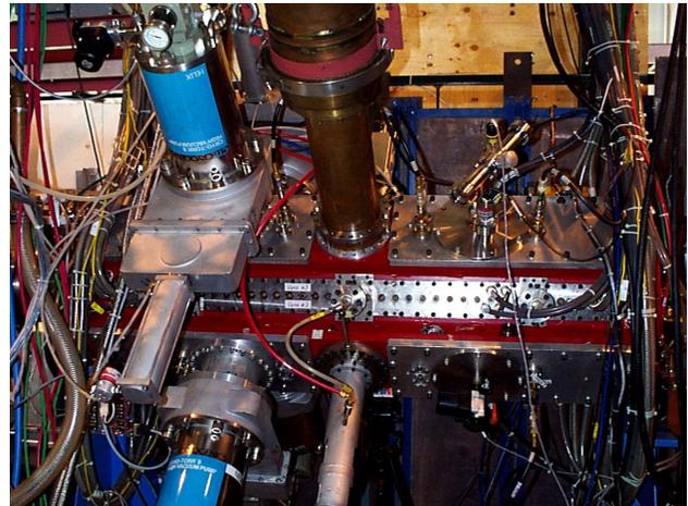
Figure 1: The CRITS RFQ accelerating structure.
