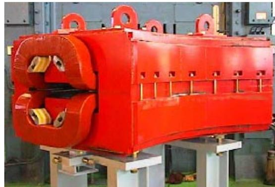
Figure 3: The prototype dipole magnet
