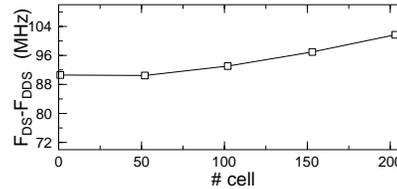
Figure 7: Frequency shift due to the damping slots.
