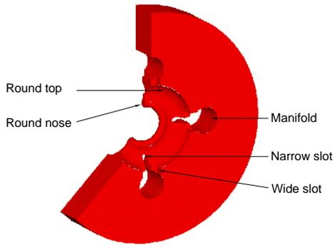
Figure 4: Damped RDDS structure cell.
