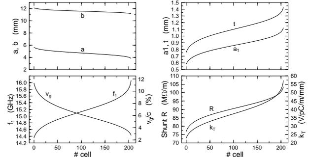
Figure 3: RDS structure cell dimensions and rf parameters.
