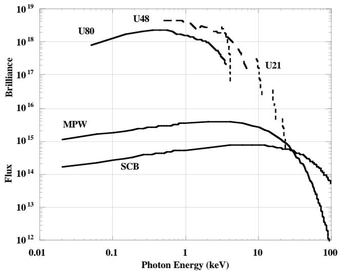
Figure 4: Flux (ph/sec/0.1% bandwidth) for the multipole wiggler (MPW) and superconducting dipoles (SCB); Brilliance (flux/mm<sup>2</sup>/mrad<sup>2</sup>) from the undulators.
