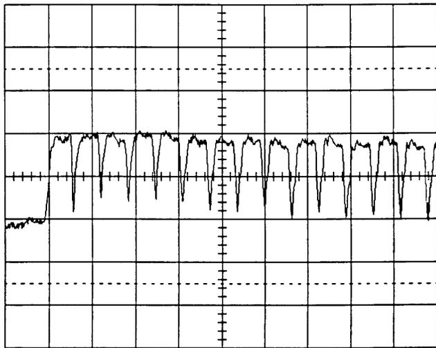
Figure 2. Current in the ring for the first several turns, using single-turn injection. The horizontal scale is 1 μs/div.
