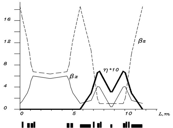
Fig.3 Machine functions of the modified TBA cell. accomplished by gradient dipole magnets, this provides the smallest value of the betatron radial function  $\beta_x$  in the
