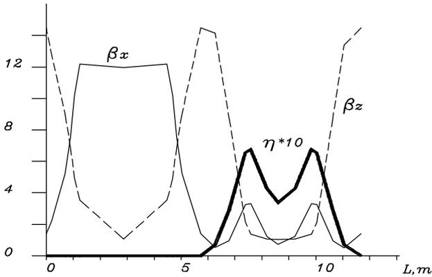
Fig. 2. The machine functions of a superperiod.
