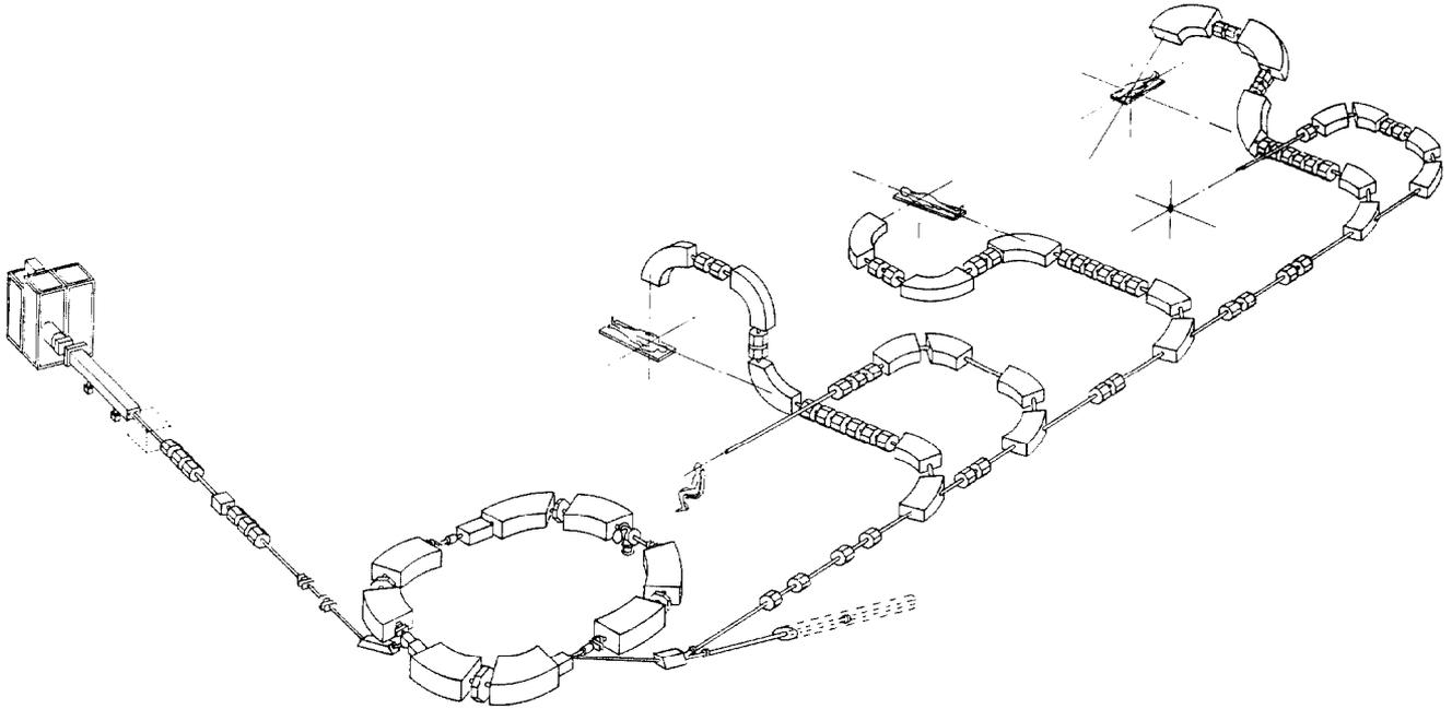
Figure 3: Isometric diagram showing the treatment facility beam lines and beam line magnets.
