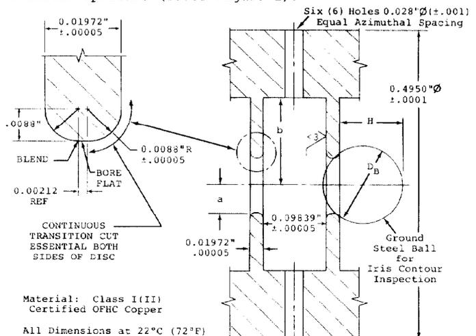
Figure 1. Cavity Details for 33.3 GHz,  $2\pi/3$  Mode,  $v_p = c$  Waveguide.
