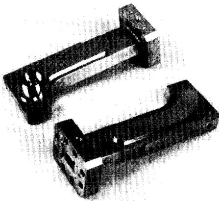
The tapered transitions had highly polished internal surfaces; and the cross-section dimensions in the E-field plane (and orthogonal to this plane) varied from .4000" (x.2800") at the oversize WR28 flange, to 0.0984" (x0.2800") at the accelerator coupler interface.
