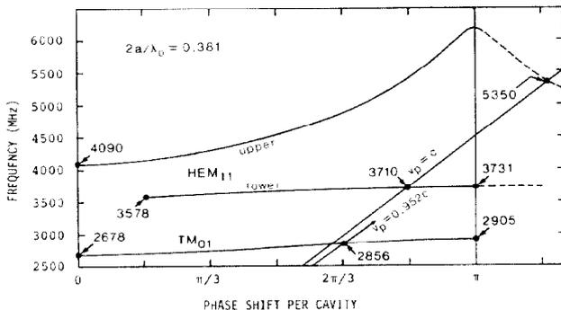
Figure 4. RF Cavity Propagation Characteristics.
