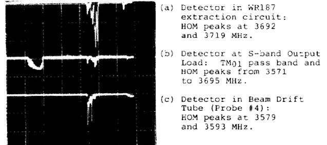
Figure 6. HEM<sub>11</sub> Frequency Transmission into External Loads.
