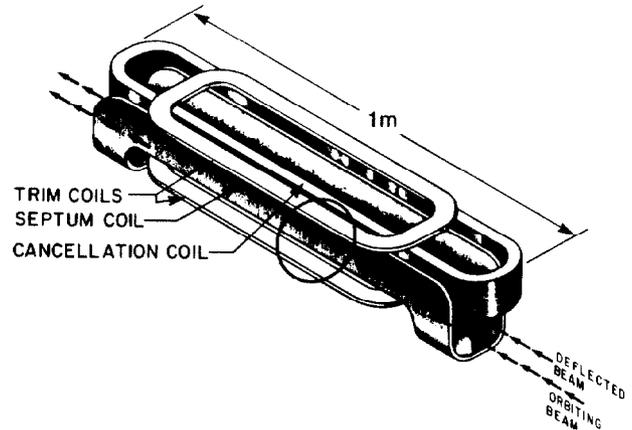
Fig. 1. An isometric view of the prototype magnetic channel. A cross section through the coils (circle) is shown in Fig. 2.
