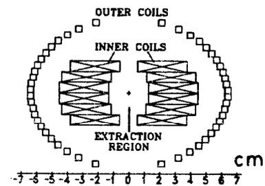
Fig. 7. A cross section through the coaxial channel, 1.3 and 0.6 kA, in the inner and outer coils respectively produces  $B_z$  of 0.3 T.
