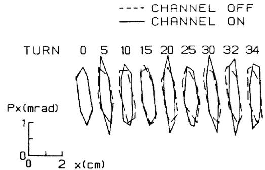
Fig. 4. Ellipses in radial phase space plotted every 5 turns (at the azimuth of the channel) as the beam passes through the leakage field. Turn 32 is the closest orbiting beam to the septum, and turn 34 is the extracted beam. Ellipses from calculations made without the channel field have been superimposed for comparison.
