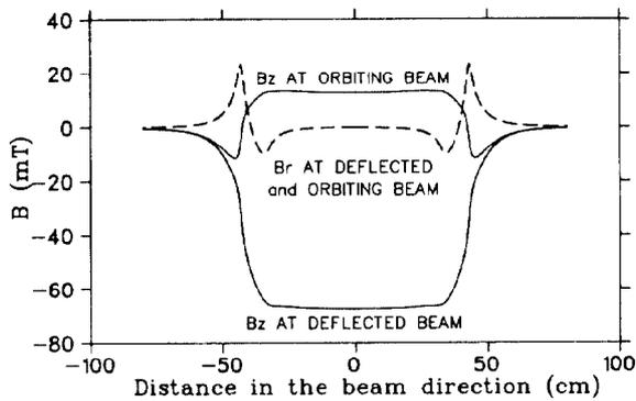
Fig. 3. The  $B_z$  and  $B_r$  components of the field experienced by the orbiting and extracted beams.
