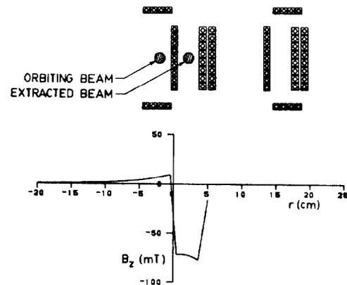
Fig. 2. A cross section through the channel used for the two-dimensional field calculation. The  $B_z$  field produced by the channel in the median plane is also shown. Currents in the coils are septum  $-700$  A, cancellation  $+480$  A, trim  $-120$  A.
