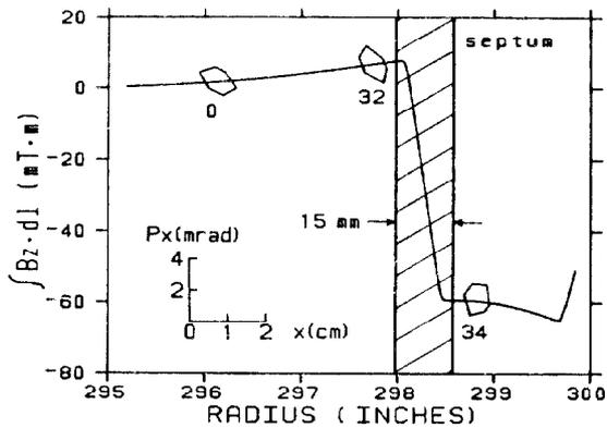
Fig. 5. Position of the septum with respect to the orbiting and extracted beams. The azimuthally integrated  $B_z$  field of the channel is superimposed.
