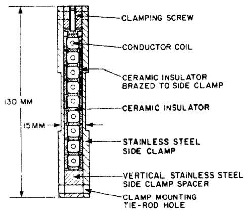
Fig. 6. A cross section through one of the radiation-resistant clamps which hold the septum conductors in place.
