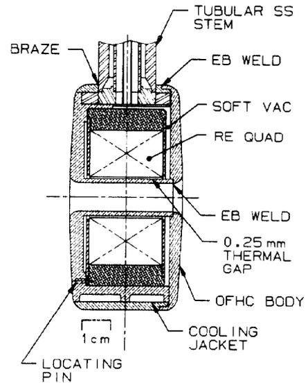
Fig. 4. Noninstrumented drift-tube body.
