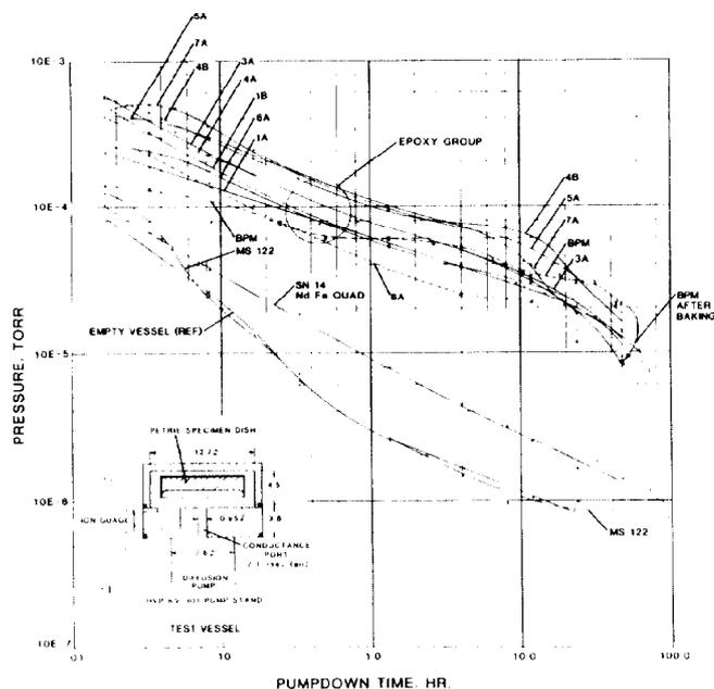
Fig. 6. Pump-down characteristics of high vacuum-grade epoxies.
