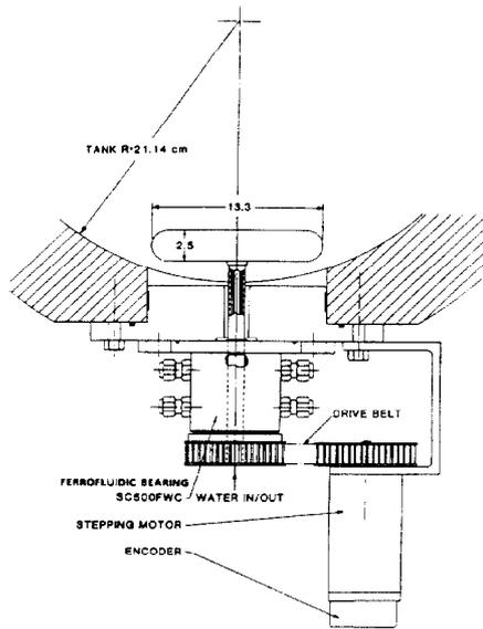
Fig. 3. Rotary tuner concept.
