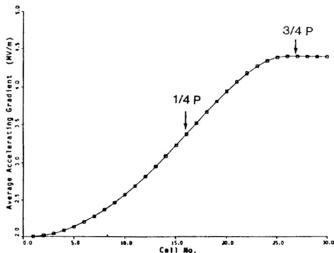
Fig. 2. Average accelerating gradient vs cell number, cubic ramp 2.0 to 4.4 MV/m over 150 cm, 3° face angle.
