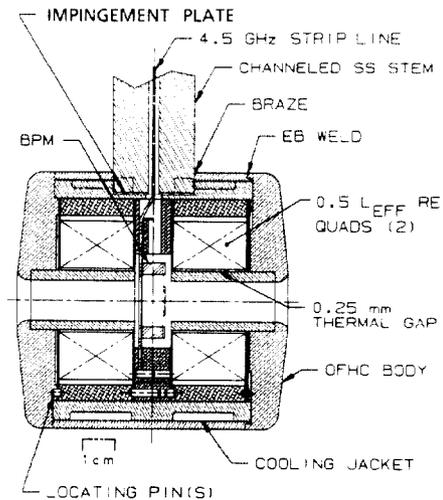
Fig. 5. Instrumented split-quadrupole drift-tube body.
