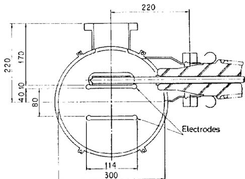
Fig. 2 Assembly of electrodes, heat pipe type bushing and a separator chamber.
