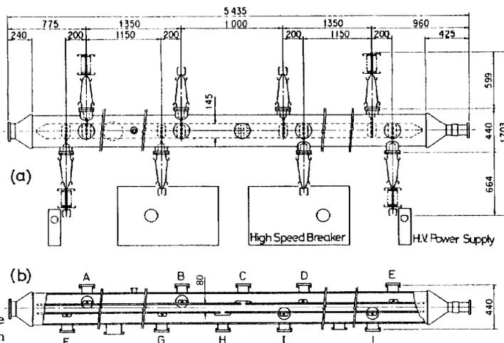
Fig. 3 (a) Assembly of high voltage bushings (L type), (b) Arrangement of electrodes.
