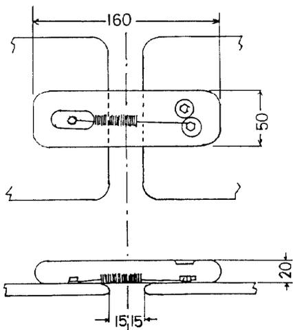
Fig. 4 Connecting part between two pieces of an electrode. Fig. 3(b), (C and H).
