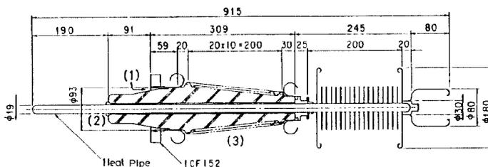
Fig. 1 High voltage bushing equipped with a heat pipe.
