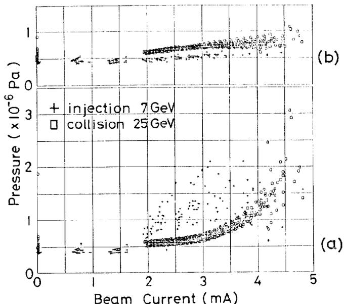
Fig. 5 Pressure change with beam current, (a) the deteriorated, and (b) normal separators.
