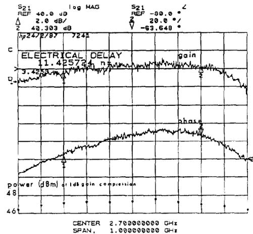
Fig. 4 - Frequency response of a power amplifier.
