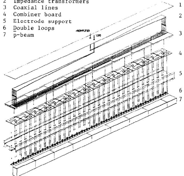
Fig. 3 - Blown-up view of a signal combination structure
