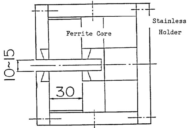
Fig.1 Cross Section of Kicker Magnet
