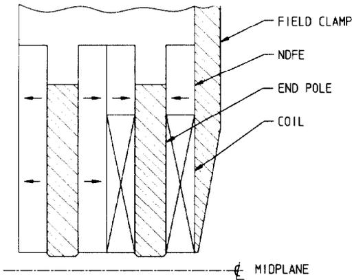
Figure 2. End Pole Configuration
