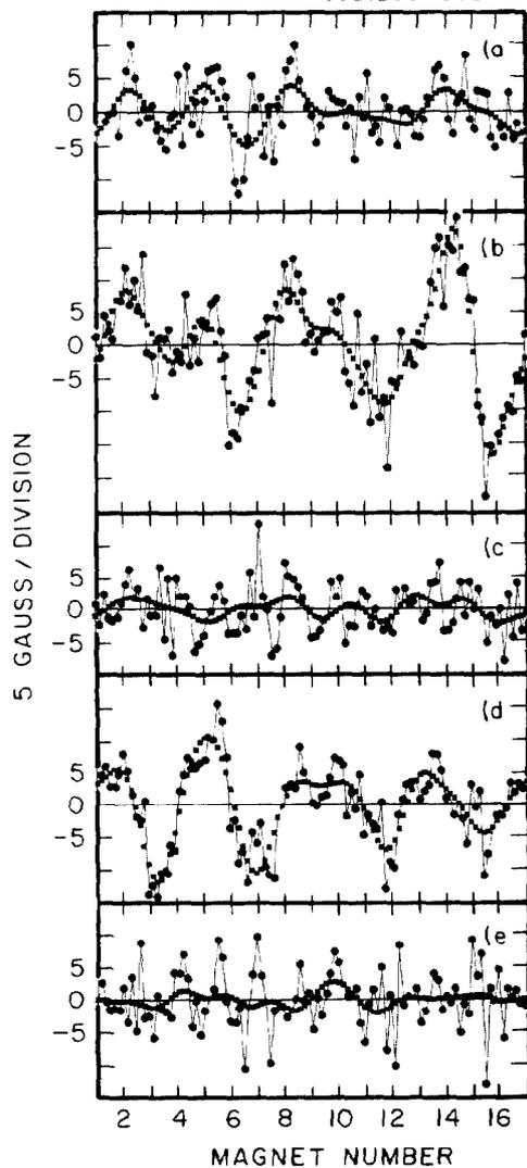
Fig. 4 Measured radial magnetic field at 4 cm radius for module #10 after subtraction of dipole and quadrupole terms, plotted vs. azimuth (magnet # 1-16). The conditions are: a) after initial tuning, b) after heating to 120°C, c) after replacing magnet #15, re-heating, and retuning, d) after exposure to a 15.5 kG axial field, and e) after retuning and final exposure to 15.5 kG. (■) includes multipoles  $n=3$  through  $n=10$  even and (●) includes  $n=3$  to  $n=50$ .
