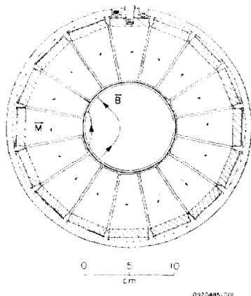
Fig. 1 Schematic of quadrupole module showing directions of magnetization and representative field lines. The shaded material is stainless steel.
