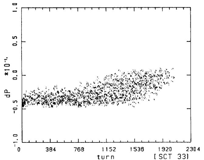
Fig. 5. Momentum deviation of the extracted beam from 30.9 GeV vs. turn number for chromatic extraction.
