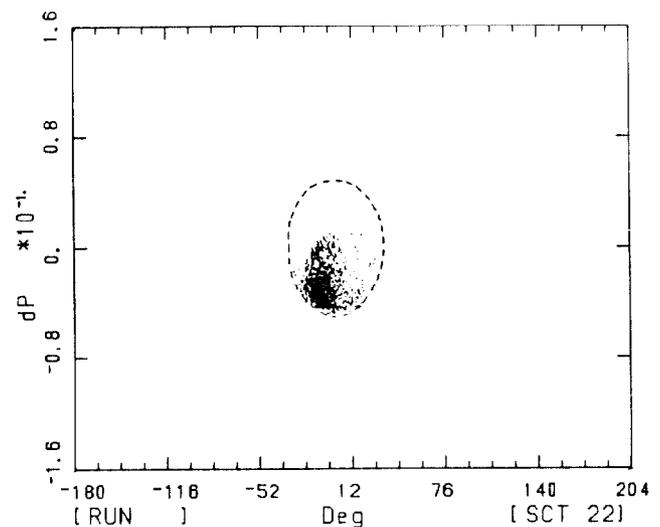
Fig. 6. Longitudinal phase space of extracted beam. Momentum deviation from 30.9 GeV/c is plotted vs. phase angle. The dashed oval is the area occupied by the circulating beam.
