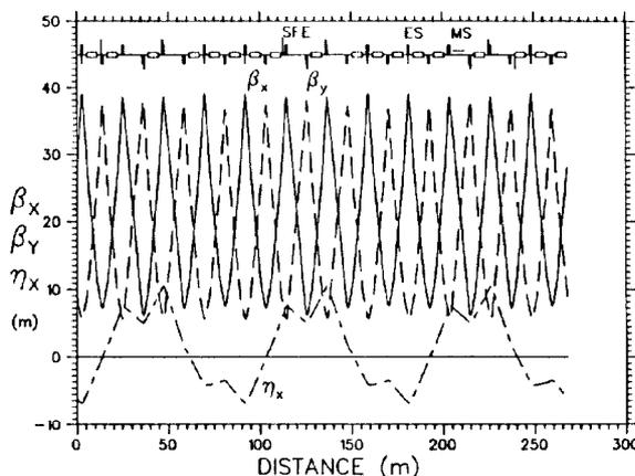
Fig. 1. Extraction elements in the Extender lattice. SFE is a sextupole, ES, MS are septa.
