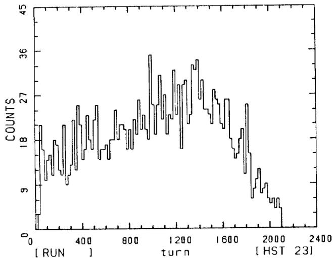
Fig. 4. Macroscopic time structure of the extracted beam for achromatic extraction.
