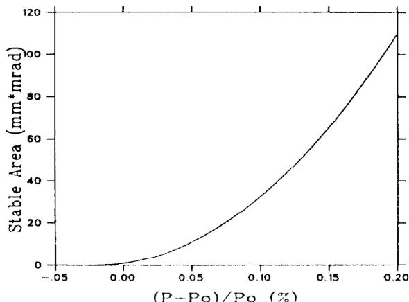
Fig. 2. Stable area as a fraction of beam momentum for natural chromaticity. Area of the circulating beam is 15 mm-mrad.
