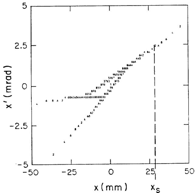
Fig. 3. Area of stability and separatrices in horizontal phase space. The septum is indicated by  $x_s$ .
