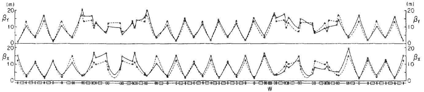
Fig. 3 Measured  $\beta$  functions in the normal optics with the VW excited (—) and not excited (---).
