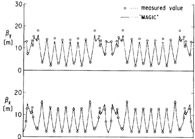
Fig. 2 Measured  $\beta$  functions of the normal optics.
