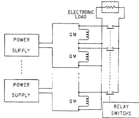
Fig. 1 Schematic diagram of shunting circuits.
