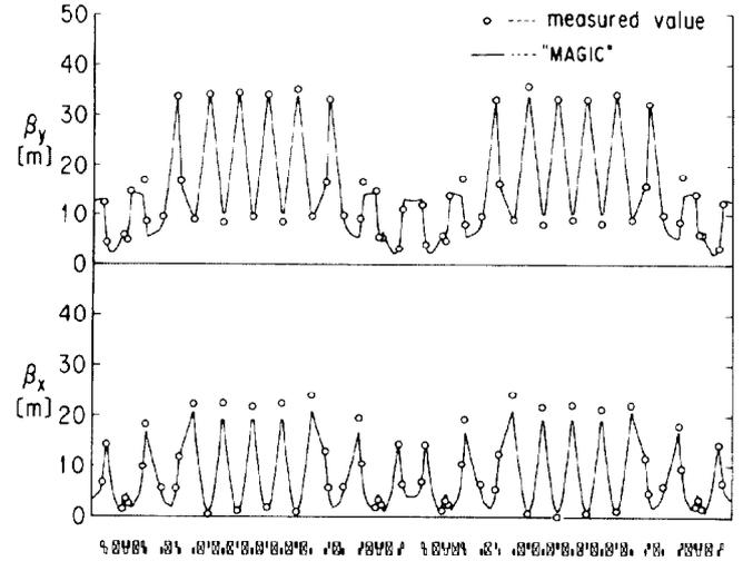
Fig. 8 Measured  $\beta$  functions of the low  $\epsilon$  optics.
