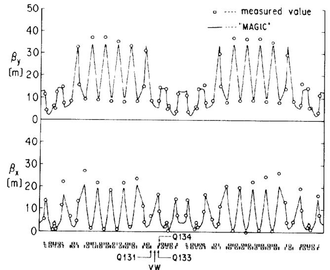
Fig. 9 Measured  $\beta$  functions of the low  $\epsilon$  optics with the VW excited to 5.0 T.
