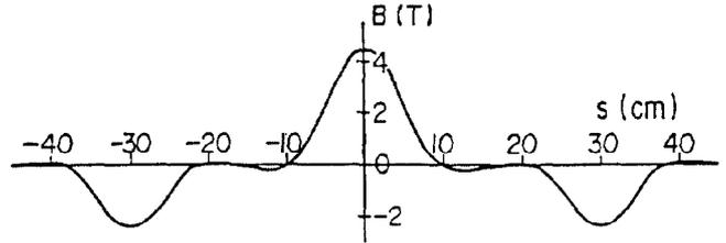
Fig. 4 Horizontal magnetic field in the VW.
