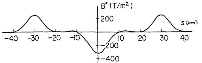
Fig. 6 Sextupole field component in the VW.
