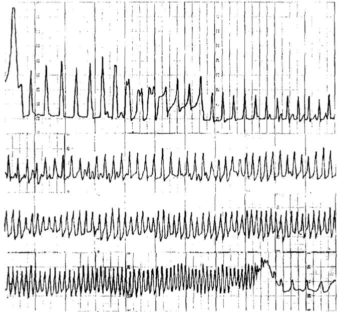
Fig. 3 The turn pattern of a 40 MeV proton beam when the cyclotron magnetic fields were exactly the same as the calculated fields. This figure shows the turn pattern from the position where the first phase selection slit is in place (18<sup>th</sup> turn) to the beam extraction point. It can be seen that the turns are well separated all along the radius and there is no indication of the precessional motion of the orbit center.
