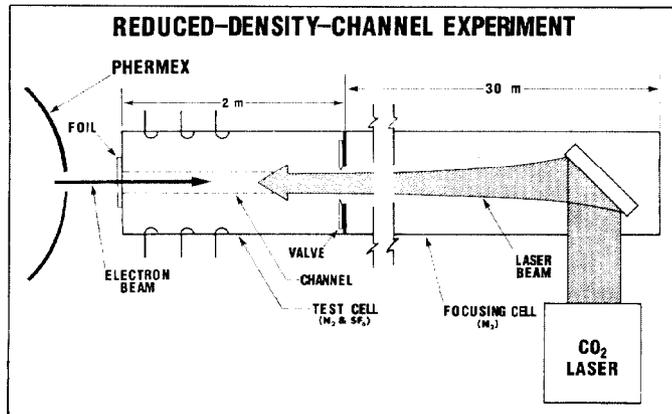
Fig. 1. Schematic of RDC propagation experiment.
