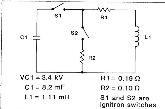
Fig. 5. Simplified electrical schematic with the capacitor bank and field coils.
