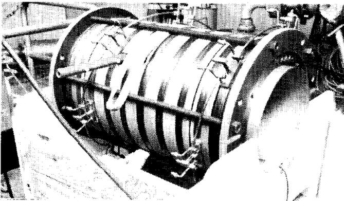
Fig. 4. Photograph of the magnetic field coil assembly.
