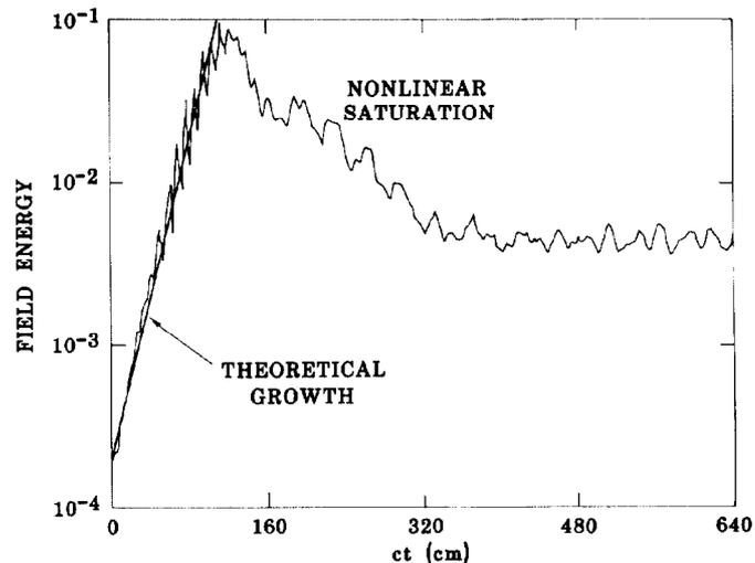
Figure 4. Energy in  $k = 0.3/\text{cm}$  mode relative to energy in equilibrium fields as a function of time for hydrogen ion channel.
