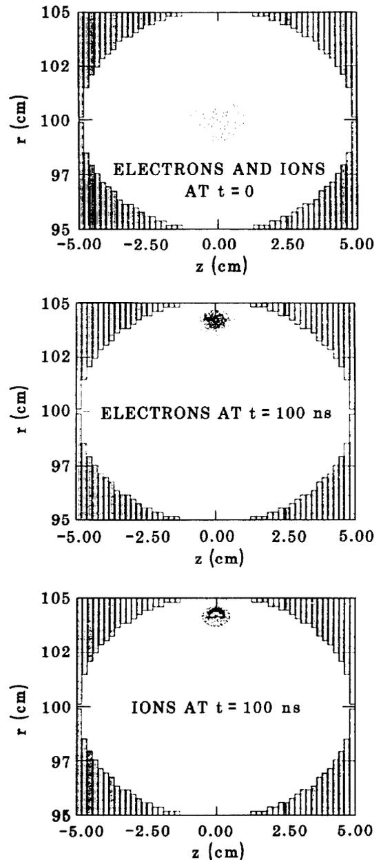
Figure 2. Decrease in beam and channel radii due to acceleration. Centrifugal force causes drift to wall.
