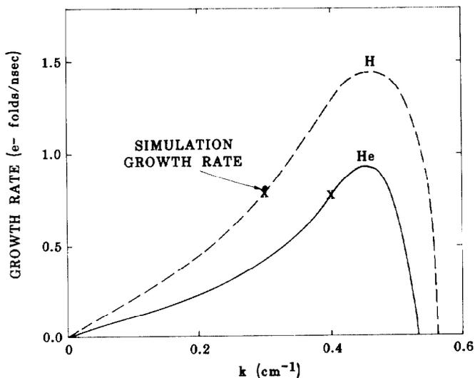
Figure 3. Growth rate versus axial wavenumber for ion-resonance instability for 15 kA,  $\gamma = 4.6$ ,  $f = 1/2$ ,  $a = 1$  cm. "X's" mark modes simulated with IVORY.
