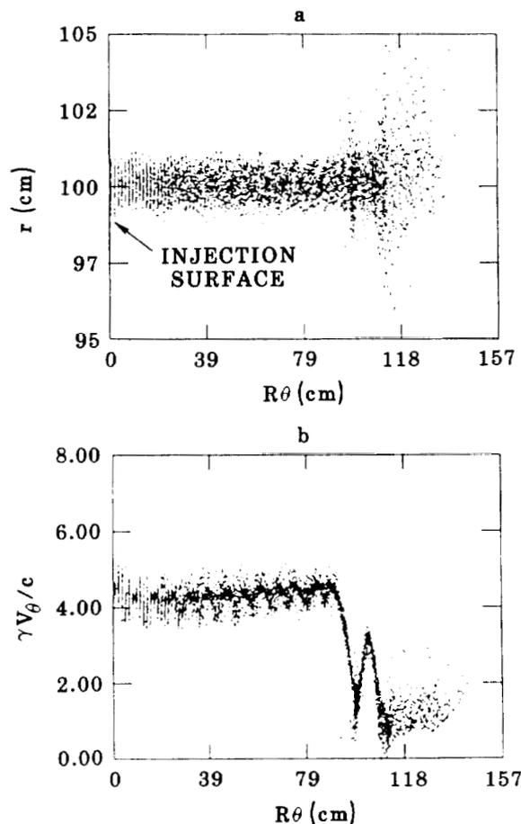
Figure 1. Particle plot from 15 kA, 2.5 MeV injection simulation at time  $ct = 200$  cm. Only the beam electrons are shown. Particle positions are shown in (a) and axial momenta are shown in (b).  $\theta$  is toroidal angle.
