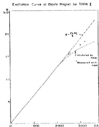
Fig. 3 Excitation characteristics of the dipole magnet for TARN II.
