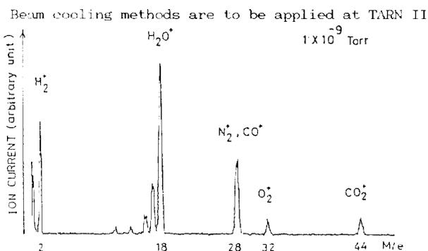
Fig. 8 Residual gas spectrum of the dipole chamber.
