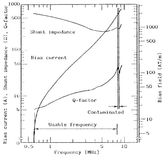
Fig. 7 Results of low-level measurement of RF cavity.
