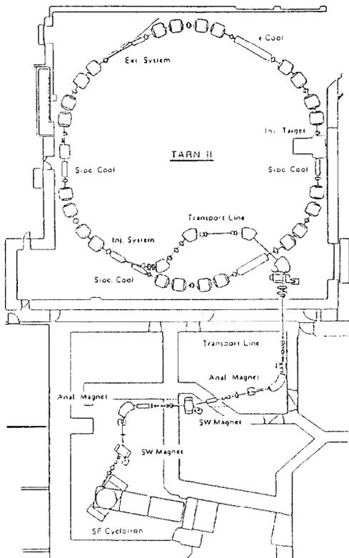
Fig. 1 Layout of TARN II and its transport line.
