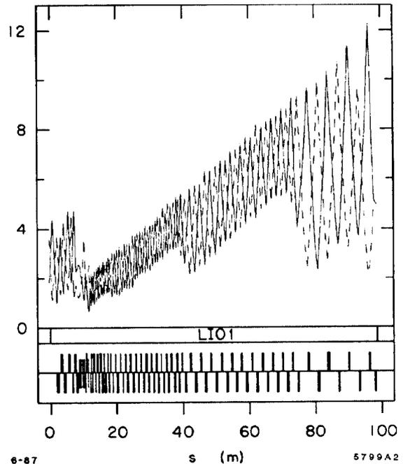
Fig. 3. Typical Twiss parameter display showing beamline elements in iconic form at the bottom.
