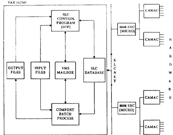
Fig. 2. Functional diagram showing how modeling fits into the SLC control system environment.
