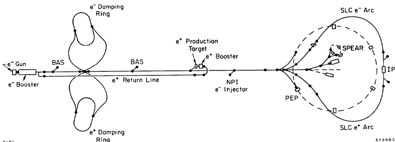
Fig. 1. Schematic layout of SLAC complex showing modeled areas (solid lines) and treaty points (dots).
