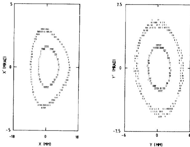
Fig. 7 Phase space plots from tracking 400 turns.
