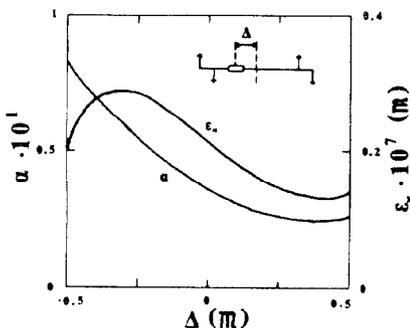
Fig. 8 Effect of changing dipole position in doublet cells.
