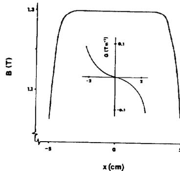
Fig. 9 Field homogeneity in dipole at  $1.3 \text{ T}$
