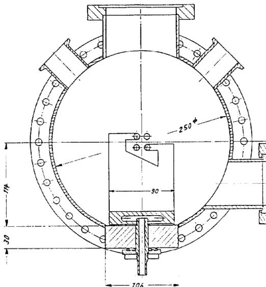
Fig.2 Cross-section of the four-rod resonator
