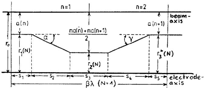
Fig.3 Parameters of the trapezoidal rod modulation
