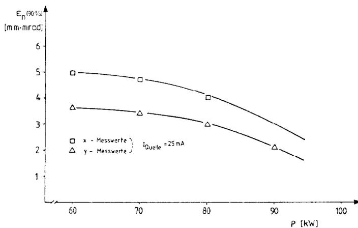
Fig.10 Measured beam emittances vs. rf power
