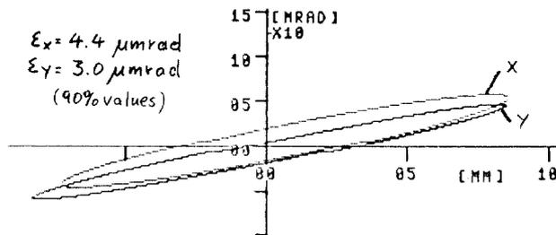
Fig.9 Emittances in x- and y-plane (80KW, 25mA)
