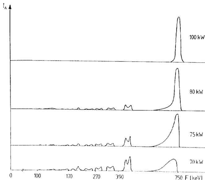
Fig.7 Energy spectra for different rf powers
