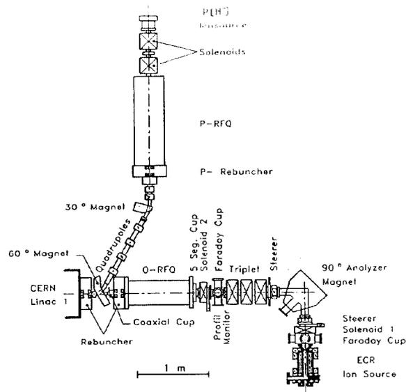
Fig. 2. Proton and oxygen injector for CERN Linac I.
