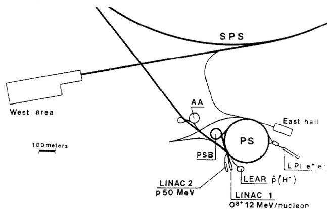
Fig. 1. Layout of the accelerator complex for the  $^{16}\text{O}$  beam. The North Area with its beam transfer line (not shown) is located  $120^\circ$  clockwise around the SPS from the transfer line to the West Area. AA, LEAR and LPI are not involved.
