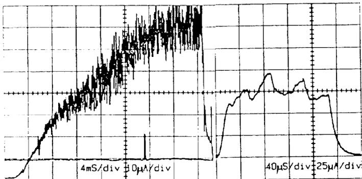
Fig. 3.  $O^{6+}$  beam from source. | Fig. 4.  $O^{6+}$  beam from RFQ.
