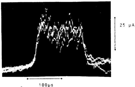
Fig. 5. The  $O^{8+}$  beam in LI-PSB line; 4 pulses superimposed.
