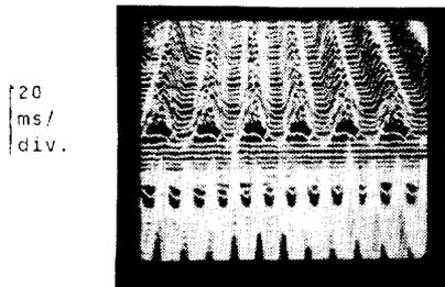
Fig. 6. PSB acceleration including the debunching, rebunching process ( $h=10 \rightarrow 5$ ). The scans start at 140 ms after injection.
