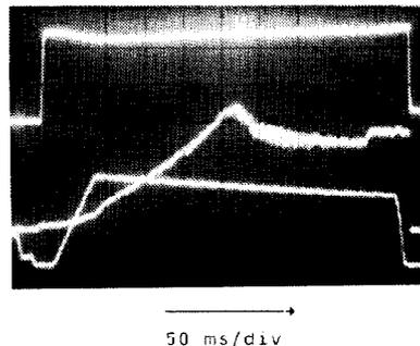
Fig. 7. Signals from the beam current transformer (top), and the wide-band PU, as well as dB/dt (bottom) during one PS cycle.
