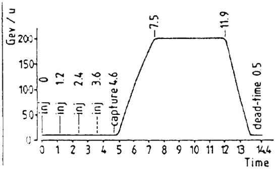
Fig. 8. SPS cycle of 14.4 s. duration for the acceleration of  $10^{10}$  oxygen ions to 200 GeV/u with 4 batch injection and a flat-top length of 4.4 s.
