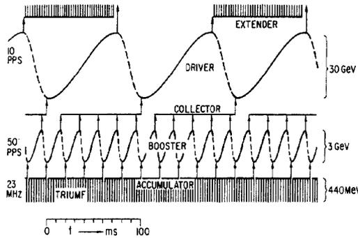
Fig. 6 TRIUMF II facility operation.
