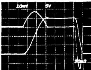
Fig. 11c Long flat-bottom, "slow" current rise, long flat-top and "fast" current decay.
