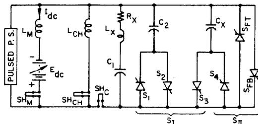
Fig. 8 Proof-of-concept SCR circuit.
