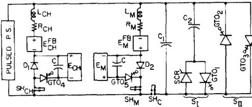
Fig. 10 Proof-of-Concept SCR and GTO circuit.
