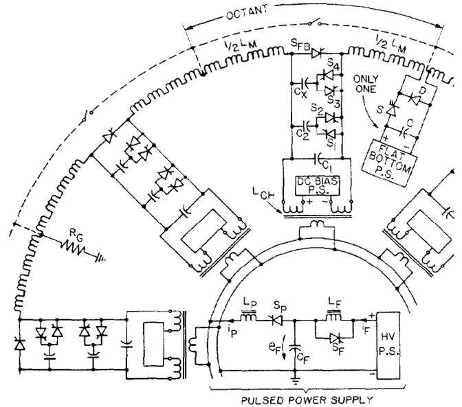
Fig. 12 RMPS for LAMPF II 6 GeV 60 pps Booster.
