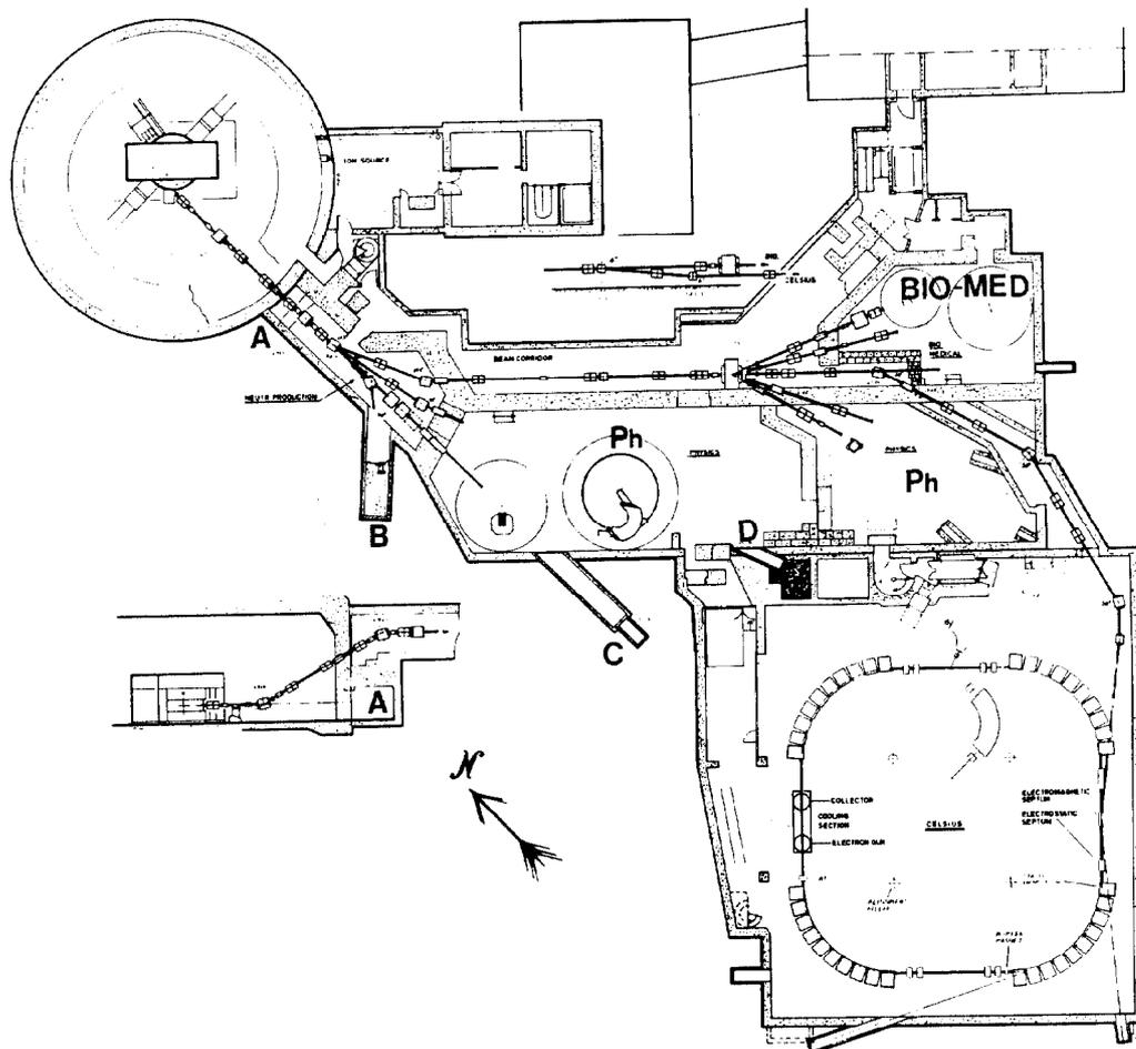
Fig. 2. Floor plan of the cyclotron hall with the rebuilt Gustaf Werner Cyclotron, new external beam experimental areas for physics (Ph) and biomedical research (BIO-MED), and the 1000 m<sup>2</sup> hall for the CELSIUS storage ring. (A), (B), (C) and (D) indicate possible sites for parasitic production of radionuclides. (From the GWI Drawings Office. Reproduced with permission from the GWI Info-Dept.)
