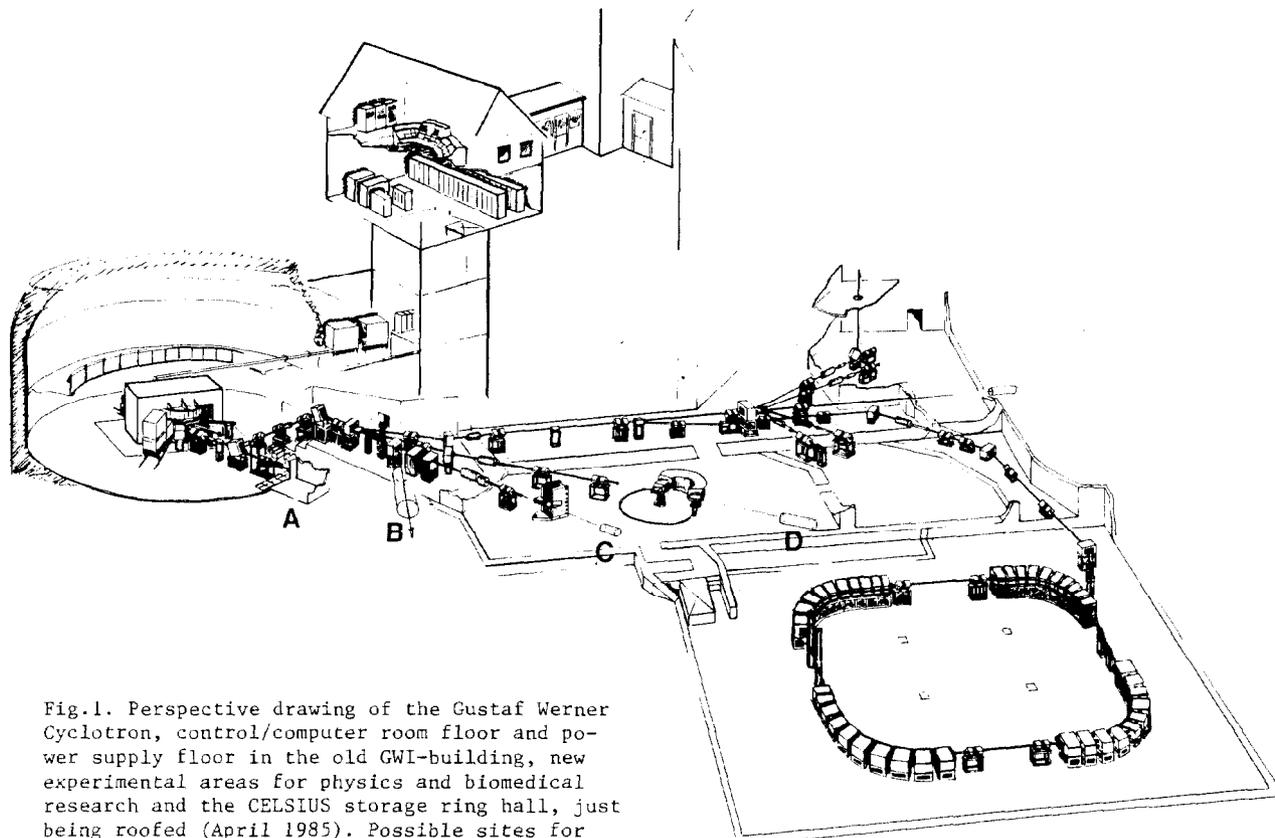
Fig.1. Perspective drawing of the Gustaf Werner Cyclotron, control/computer room floor and power supply floor in the old GWI-building, new experimental areas for physics and biomedical research and the CELSIUS storage ring hall, just being roofed (April 1985). Possible sites for parasitic production of radionuclides are indicated by (A), (B), (C) and (D). (Drawing by O. Byström. Repr.w.perm.fr.the GWI Info.dept.).
