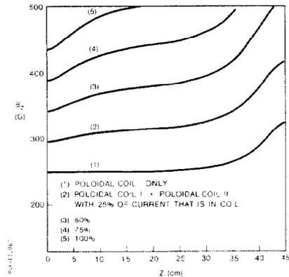
Fig. 3. Axial magnetic field at the location of the electron beam for increasing values of poloidal field II (mirror compression field).
