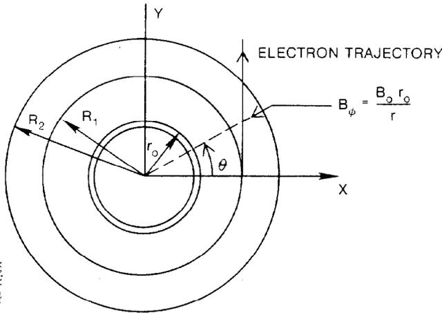
Fig. 5. Calculation of electron trajectory modification due to toroidal field by the midplane Z is illustrated  $r_0$  = initial beam radius (6 cm);  $R_1$  = radius at which the beam is extracted (12 cm); and  $R_2$  = radius of the toroidal return conductor (21 cm) beyond which  $B = 0$ .
