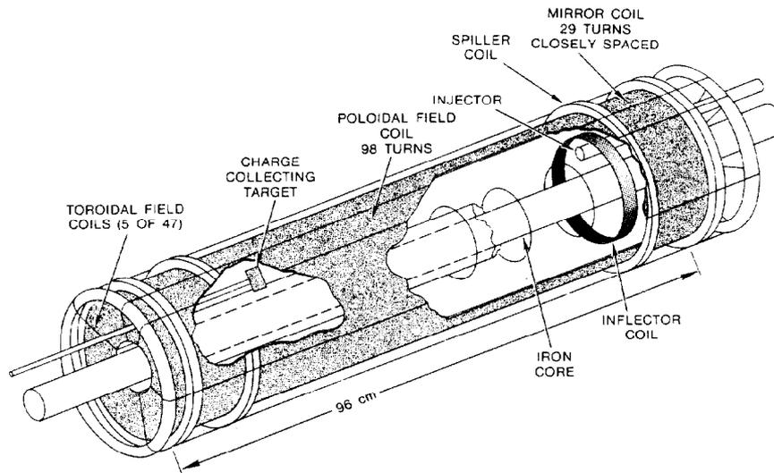
Fig. 1. Drawing of Modified Elongated Betatron Accelerator (MEBA) showing the accelerator magnetic field geometries and charge diagnostic.
