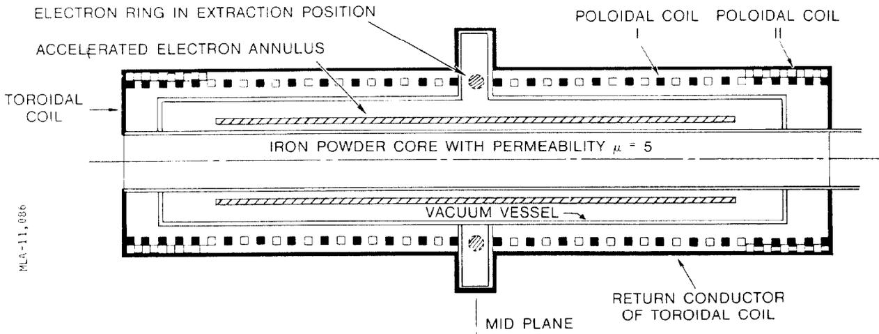
Fig. 2. Schematic diagram of MEBA accelerator with auxiliary coils for bunching and extraction.
